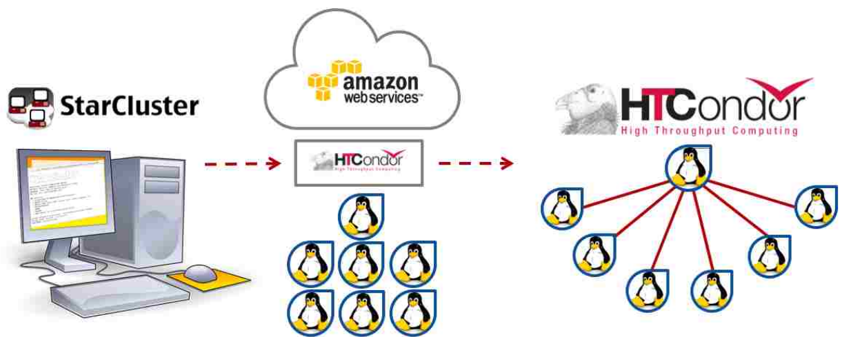
Figure 2-16 Diagram of How Starcluster, AWS, and HTCondor Interact
