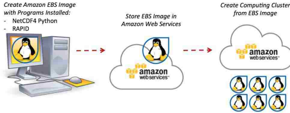
Figure 3-6 Diagram of Creating and Using EBS Image
